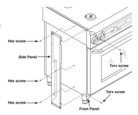
Use the hex head screw (83023) removed from the side, a Torx head screw removed from the kick panel and the hex screws from the kit to attach the side panel to the range. Three (3) hex head screws attach the side. One (1) Torx head screw (83709) inserts through the end cap hole to attach the top of the side panel. One (1) Torx head screw (83709) inserts through a hole in the front panel to attach the bottom of the side panel.
